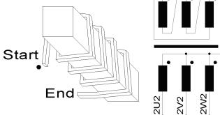
Usual manner of the inter connection from the coils for a Delta Star vector group and the connections from the transformer clamps L1, L2, L3 to the clamps L1, L2, L3, from the TSRD, when windings are put on in a clockwise manner onto the Iron core, if looking to the top of the coil and to the winding start, for a DYN5 vector group transformer.
