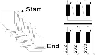
View to top of the iron core, if the coils are produced in a count clockwise manner.
